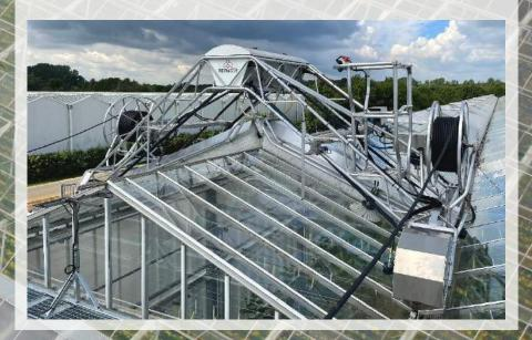
Spraying coatings is an effective way to create a better greenhouse climate, improving crop quality and production. With the Roofmaster, coatings can easily be applied and removed at those times of year it suits best.
